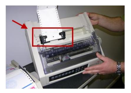
Place the form face down into the paper guards. Place the first two holes in the paper over the tractor pins on either side of the printer and close the guard covers.
