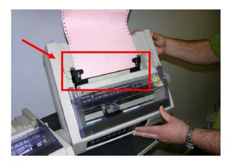
Fine-tune the position of the right tractor to center the holes in the paper on the pins, and push back the right lock lever.
